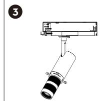
Rotate adaptor lock B clockwise 90° to connect the adaptor to the neutral circuit.
